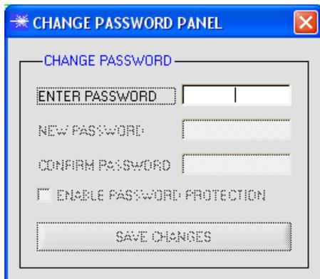
When password protection is enabled, the menu items "**File**" and "**Configuration**" only can be accessed after pressing "**Deactivate Password Protection**" and entering the correct password.
