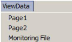
Due to lack of space only 4 sensors can be displayed on the screen. Use the **"Page1"** and **"Page2"** menu items to toggle between the first 4 and the last 4 connected sensors.
