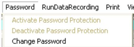
The "**File**" and "**Configure**" items can be protected by a password. Password protection can be enabled and disabled. The default password is: 0000000000 (in words: 10 zeroes). The password can be individually changed.
